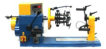
plates can be set accurately on to the armature slot edges, the axial adjustment is provided with a micrometer adjustment. The various lengths of the armature shaft are set between centres on the armature holder. The armature can be held both with and without centralization of the axis. A guide hook covers the commutator so that the wire insulation is not damaged as the armature is wound.
