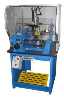
• The tailstock is provided with a ball race and quick release lever. The machine is provided with a universal winding spindle with cones for easy clamping of the bobbins.
