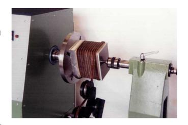
The automatic wire guide is driven by a servo motor giving infinitely variable control. Supplied with a 300mm faceplate (larger on request)
