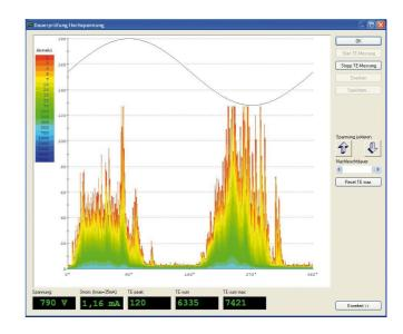
The picture shows a loose winding wire. The winding wire touches the lamination or is a small distance away from it.
