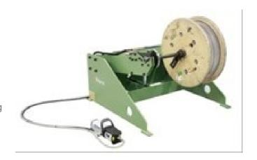
The drum is mounted to the drum shaft by means of cones to accept a range of drum hole sizes. This shaft also carries the back tension brake, comprising of a brake drum onto which a brake band operates. Tension adjustment is provided via an air cylinder connected to a pressure regulator and switch.
