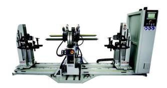
2 clamps for the stator slot length are provided. These clamps are used to hold and shape the radii of the coil during the opening phase. They are manually positioned according to the required lengths. The clamps are designed for a quick set up when changing the batch.
