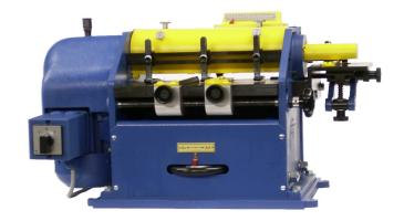
automatically by the right and left hand threaded screw with handwheel adjustment: distance between creases is shown on a scale on top of the machine.
