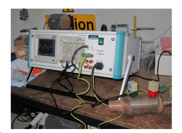
cover a wide range of rotor sizes and slot widths. The sensors are set on the rotor surface in pairs. This allows a step by step testing of each bar of the rotor and therefore precise fault determination and location. During the test there is no danger of test piece damage to the user. Sensors: 2-3 sets of probes Display unit: Digital Storage
