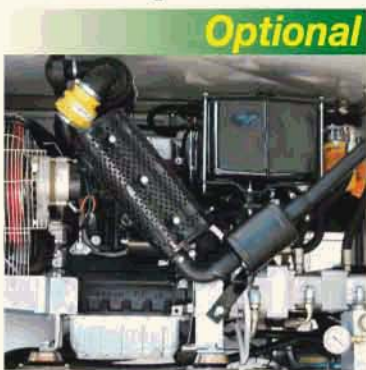
Water cooled diesel engine
