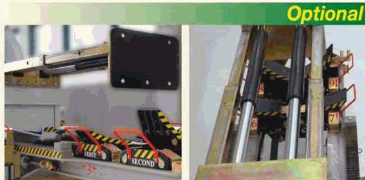
Hydraulic telescopic extended arm for bundle insertion
