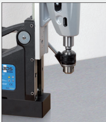
2. Place drill chuck in MT arbor.
