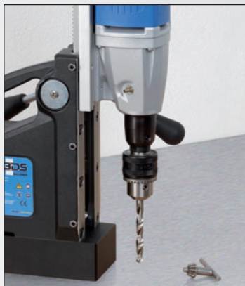
3. Ready for use with twist drill.
