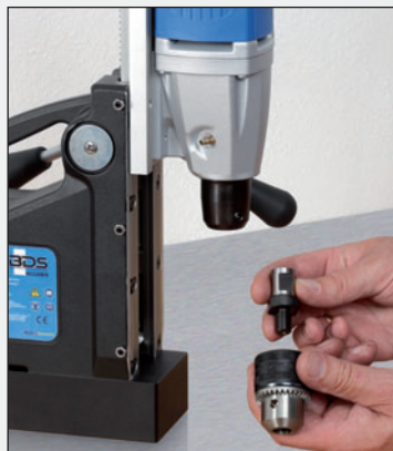
1. Connect adapter to drill chuck.
