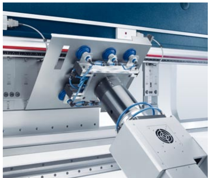
TruBend Cell 5000 with vacuum gripper.
