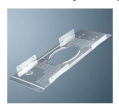
In addition to punching holes, you can produce three-dimensional contours such as brackets, threads and other forms. The electro-hydraulic punching head takes complete charge of processing your parts, eliminating the need for most downstream processing steps. Other benefits include:
