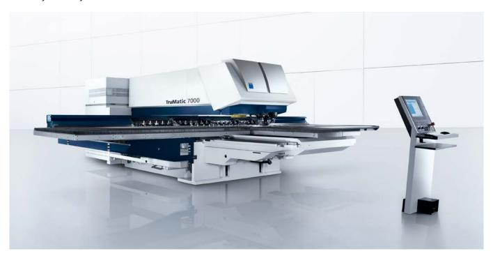
All TruMatic machines are manufactured in an open C-frame design which gives you access to both the machine and the workpiece from three sides. With this configuration there is plenty of room for both manual and automated loading and unloading. Our machines are extraordinarily stable, ensuring high levels of accuracy and a long service life.
