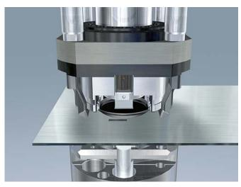
The wear-free ram guidance system combined with the mechanism that actively retracts the punch ensures accurate results and maximum process reliability.
