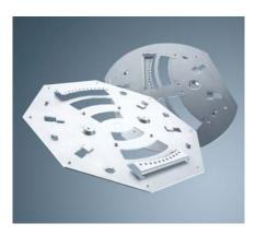
Nothing beats lasers when it comes to cutting high-grade outer contours and intricate inner contours. With the slimline laser head of a TruMatic, you can cut right next to formed areas – or even cut on top of them. ControlLine maintains a constant distance between the sheet and the cutting nozzle, resulting in a highly reliable process for fabricating even the most unusual geometries.
