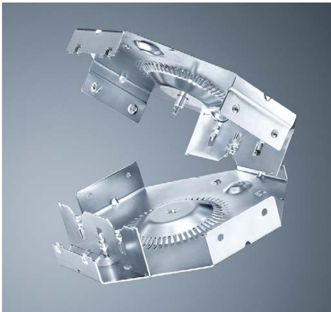
Tools and technologies used: Punching, roller deburring, forming: thread with upward and downward extrusion, upward thread punching, cup, clip and hinge, bridges, MultiBend, embossing.
