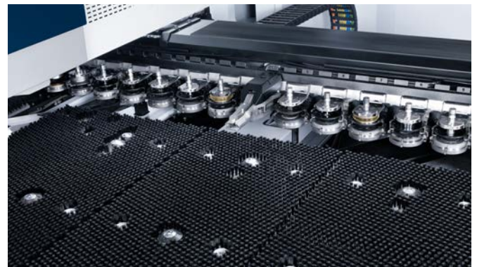
Brush tables for a gentle material handling.
