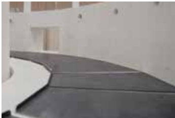
Rotary table with base plates made of highly heat-resistant steel to protect the insulation
