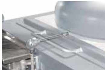
Bath control with thermocouple in the melt
