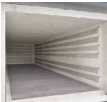
Meander shaped heating elements for short process times
