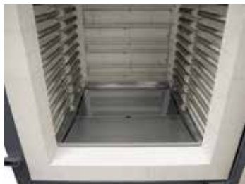
Drain pan in floor
