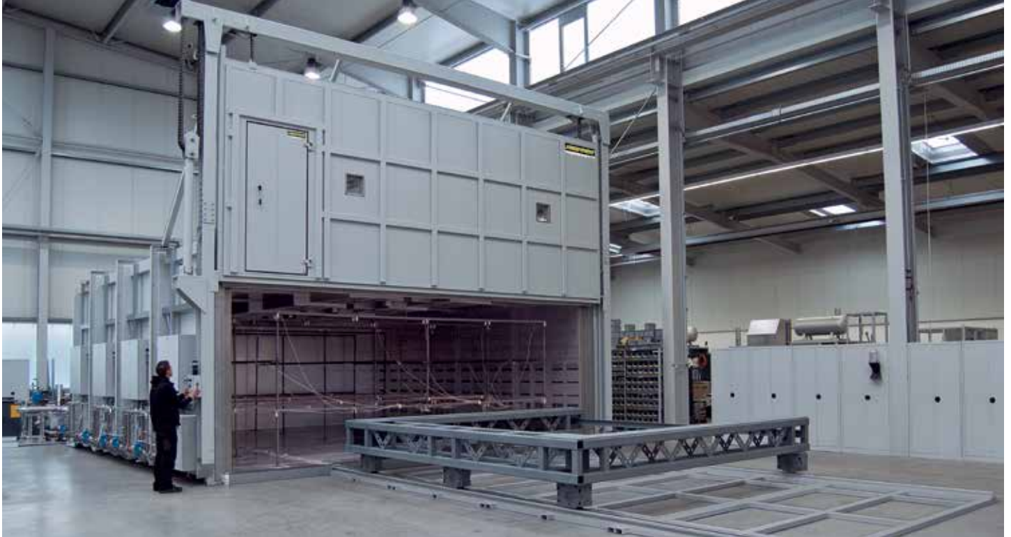
Air circulation chamber furnace N 140000/26AS for curing of composites in vacuum bags incl. pump and necessary connections in the furnace chamber
