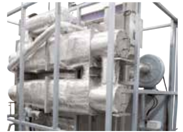
Counterflow heat exchanger for the air circulation chamber furnace N 2560/26 ACLS
