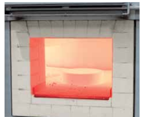
Pre-heating of steel rings for forging
