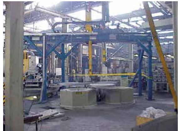
Rotary table system with 3 x T 150/11
