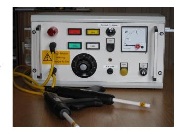
THPG-5 is supplied with test pistols but for the larger models measuring leads must be connected directly to the device under test, connection via test pistols is not possible.
